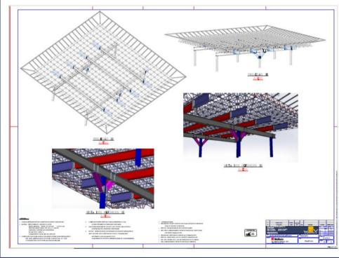
The Helipad in downtown São Paulo used to suffer from structural displacements caused by the aircraft landing and take-off operation, due to dimensioning problems aggravated by the oxidation of the bars and tubular connection nodes. JGV Engenharia indicated and designed all reinforcement measures and structural recovery of the Helipad, improving the distribution of loads in the special structure and treating pathologies, enabling the return of Helipad operations.
