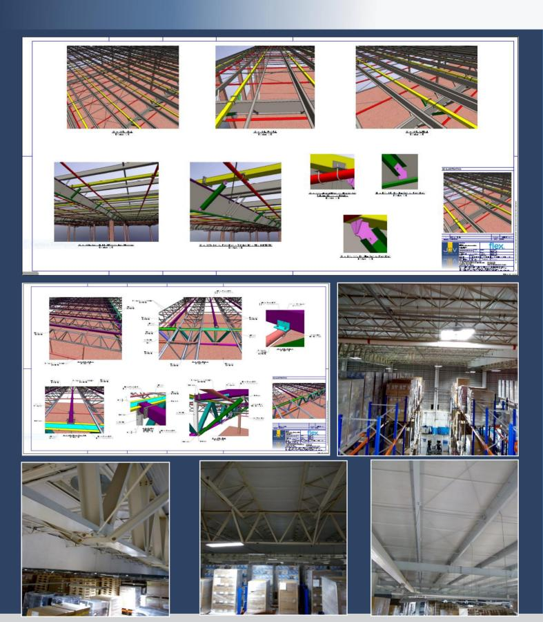
Structural reinforcement check and design for sprinkler installation disposition compliant to the FM Global standard, at the Flex factory in Sorocaba with a reinforcement line assembled to weld only in scissors, seeking savings and practicality, counting that the other pieces are all screwed. All of this in a 27,098m² area.
