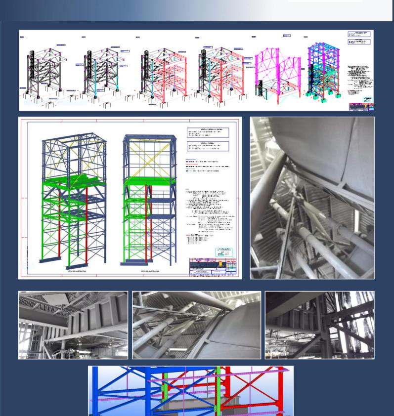
Report and Structural Reinforcement Project for the installation of two new silos in existing structure, one weighing 100 tons and the other 150 tons, at Metso Fundição in Sorocaba / SP.
