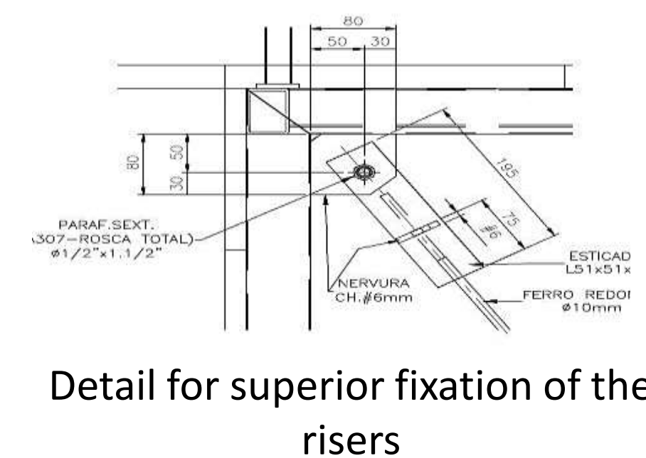
Detail for superior fixation of the risers
